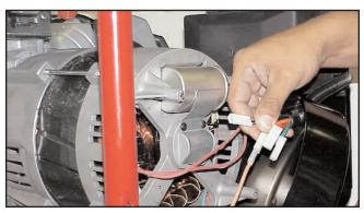
**Step 9 -** The ground lug will need to bolted to a hole on the support bar to the right of the gen - head. Torqued at 90-120 in lbs.
