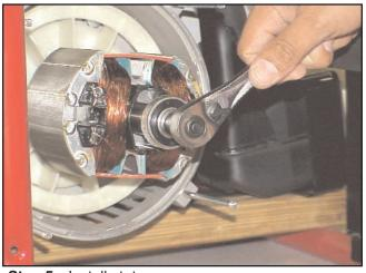
Step 5 - Install stator
