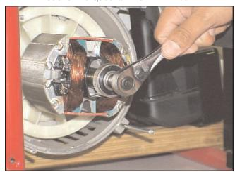
Step 5 - Install stator
