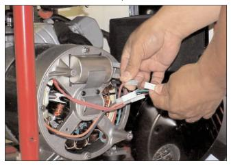
**Step 3** - Remove the grounding lug and the nuts from the isolators underneath the support bar on the frame.
