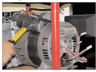
Step 5 - Remove the stator.
