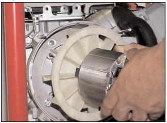
Step 4 - Install rotor thru bolt (install short threaded end of rotor thru bolt in engine shaft until threads run out), washer and nut, using a ½ socket. Torqued at 120-144 in lbs
