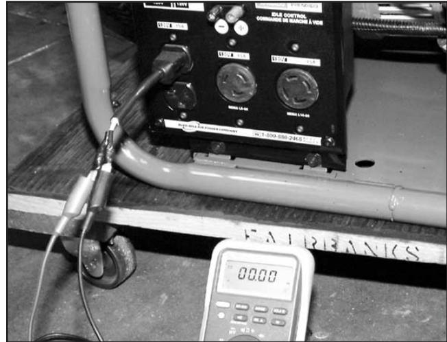
2. Using Phillips screw driver turn the screw on the carburetor left or right until the VOM (volt/ohm meter) reaches 45 Hertz. **MAKE SURE** reading remains at 45 Hertz when tightened.
