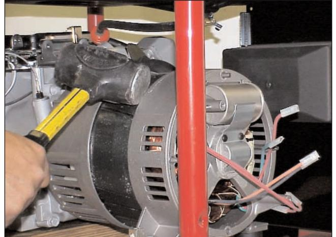
**Step 5** - Remove the stator.
