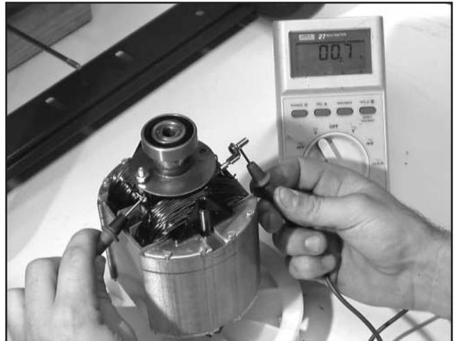
**TO CHECK ROTOR (if generator will not re-excite and Stator is OK) (cont'd)**
