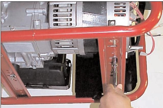
**Step 4** - Before remove the bearing support, slides a 2x4 between the engine and the frame to support the weight while working on the gen head.
